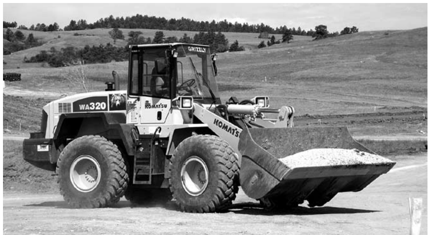
Grizzly Excavation relies on Komatsu wheel loaders for a variety of tasks, such as carrying materials and backfilling trenches. The company recently purchased this WA320-5 and rents others as needed. "The hydrostatic transmission in them is phenomenal," said Vice President Dan Earley. "They have great power and are very fuel-efficient."
