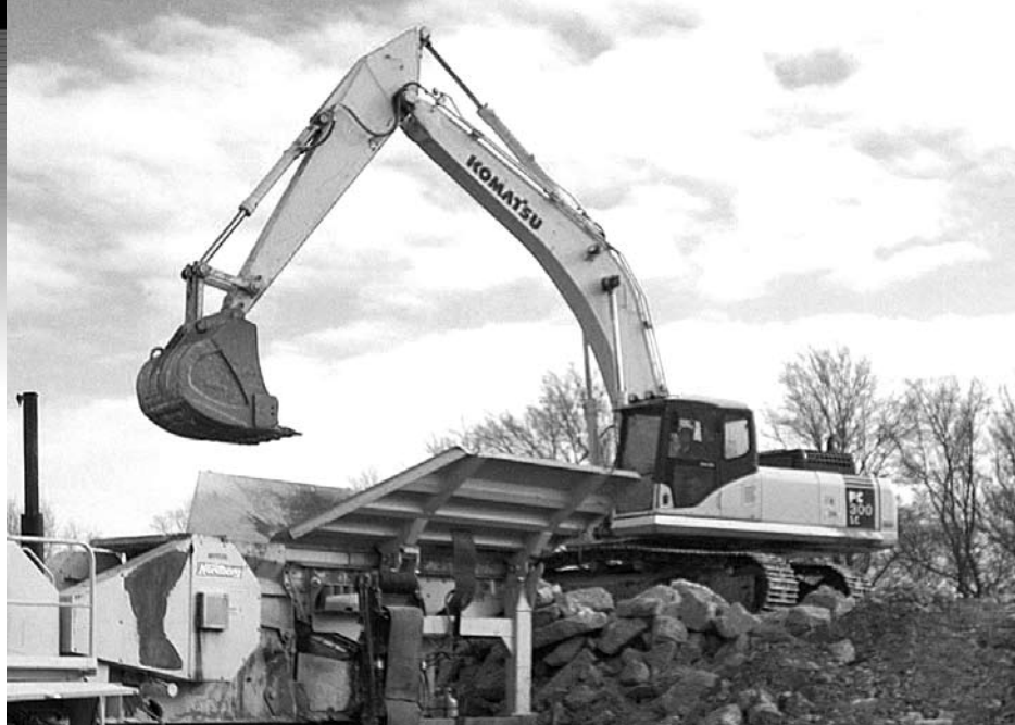
A Weatherton Contracting operator uses a Komatsu PC300LC-7 to feed a crusher. "The PC300 is excellent for feeding the crushers because its production capacity is high," said President Carl Weatherton. "Using it, we can easily feed 300 tons an hour through the crusher."
