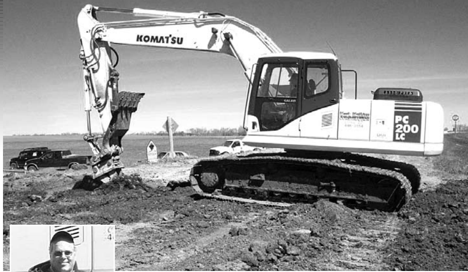
Operator Tim Basler digs with the company's PC200LC-7. "The PC200 has been a good all-around machine for us," said Owner Mark Mathieu. "We've used it for clearing, digging basements and utility trenches, loading and just about anything else you can think of, including some demolition."
