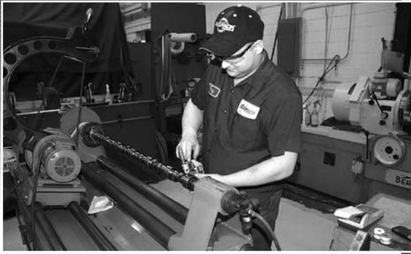
Individual parts are carefully inspected to ensure they meet OEM standards prior to being used in a reman component. Here, technician Tony Johnson measures a camshaft for a mining dozer as part of the inspection process.
