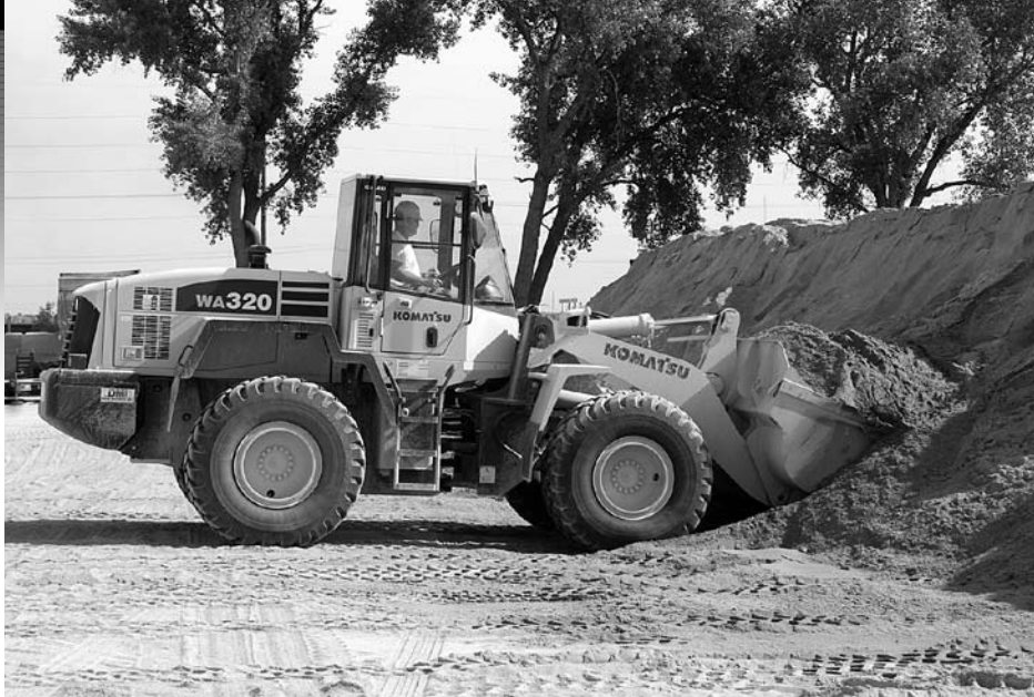
Komatsu wheel loaders are a staple in Consolidated Ready Mix's fleet, including this hydrostatic WA320-5 used to stockpile and charge the hopper at the company's concrete plant in Aberdeen. "The hydrostatic loaders have several features that make them stand out, including excellent fuel economy," said General Manager Tom Henrich.
