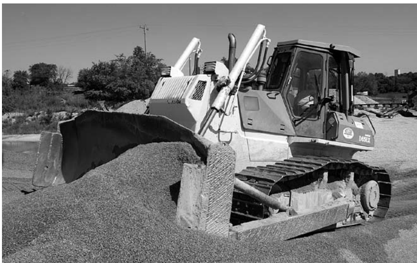
A Consolidated Ready Mix operator works on stockpiling material at the company's Big Stone City pit using a Komatsu D65 dozer.
