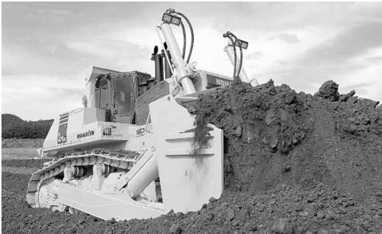
The D475ASD-5 Tier 2 dozer pushes nearly 60 cubic yards of material with its Super Dozer blade.
