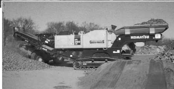
Valley Sand & Gravel, a sister company to Tri-State Ready Mix, used Komatsu excavators to break up old concrete in preparation for recycling it using a rented Komatsu BR380JG crusher.
