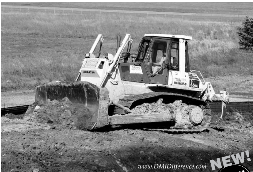
Ron Clausen moves dirt with a Komatsu D65EX-12 dozer for the building pad of a new fire station at the Watertown airport. "This D65 has about 7,000 hours on it, and we've done nothing to it other than routine maintenance and putting a new undercarriage on at about 6,000 hours," said Ron. "It's given us a very good return on investment."
