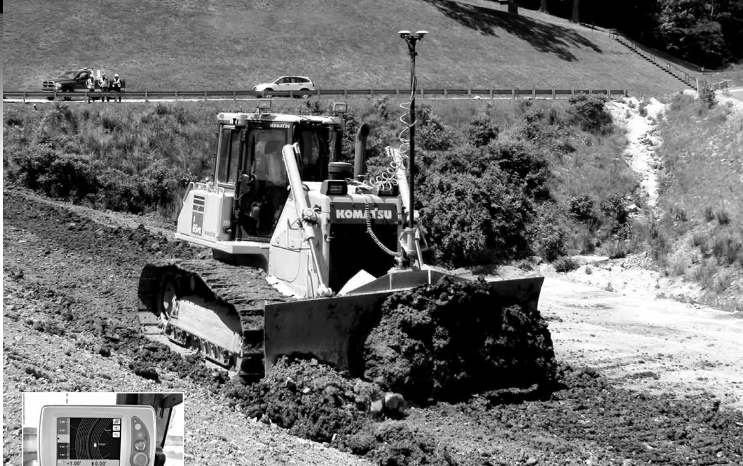
Many Komatsu models, including this D65PX, come “plug-and-play” ready for Topcon GPS systems. The Topcon 3D-MC 2 system monitor clearly shows grades and position, helping the operator get to grade faster than a manual dozer.
