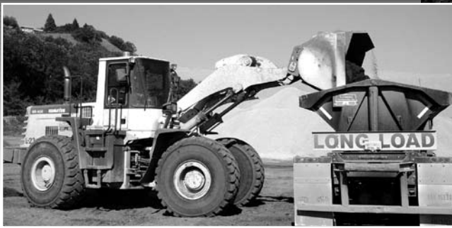
Loading trucks along Highway 52 near Yankton was easy work for this Loiseau operator using a Komatsu WA500-3 wheel loader.
