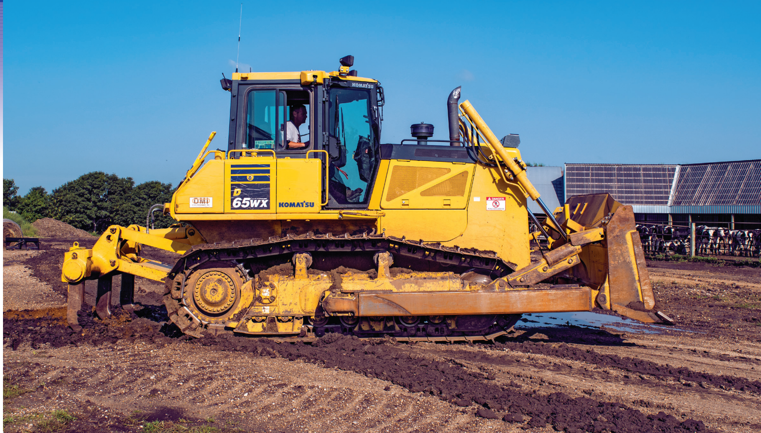
Using a multi-shank ripper on a Komatsu D65WX-17 dozer, Eric Sas, Co-owner of Sas Farms, Inc., prepares the ground for a new feeding pad at a farm near Sioux Falls. “The dozer has a lot of versatility and power to work through muddy conditions,” said Sas.
