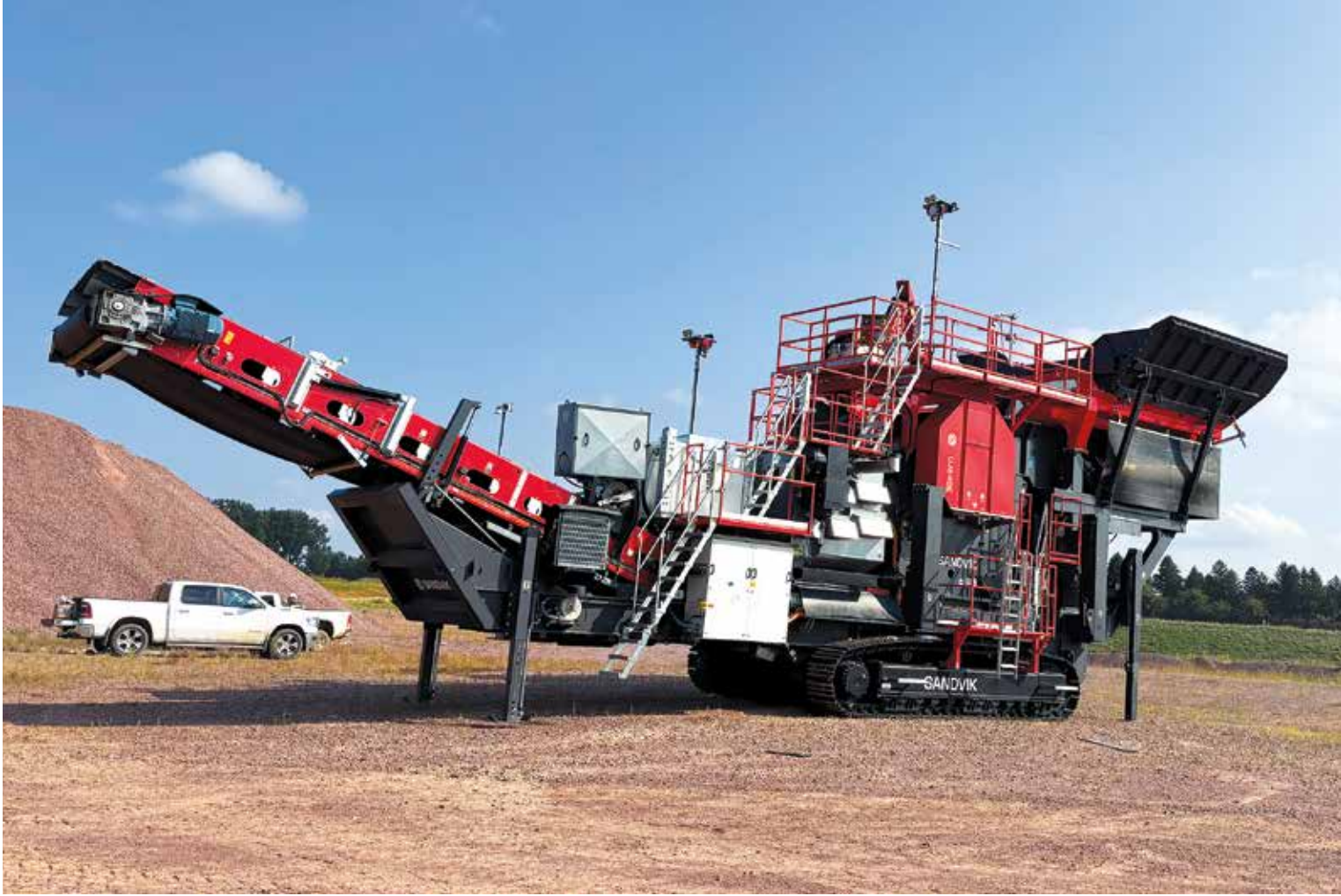
The Sandvik UJ640E tracked jaw crusher is a dual-powered unit and offers a lower cost-per-ton alternative to diesel.
